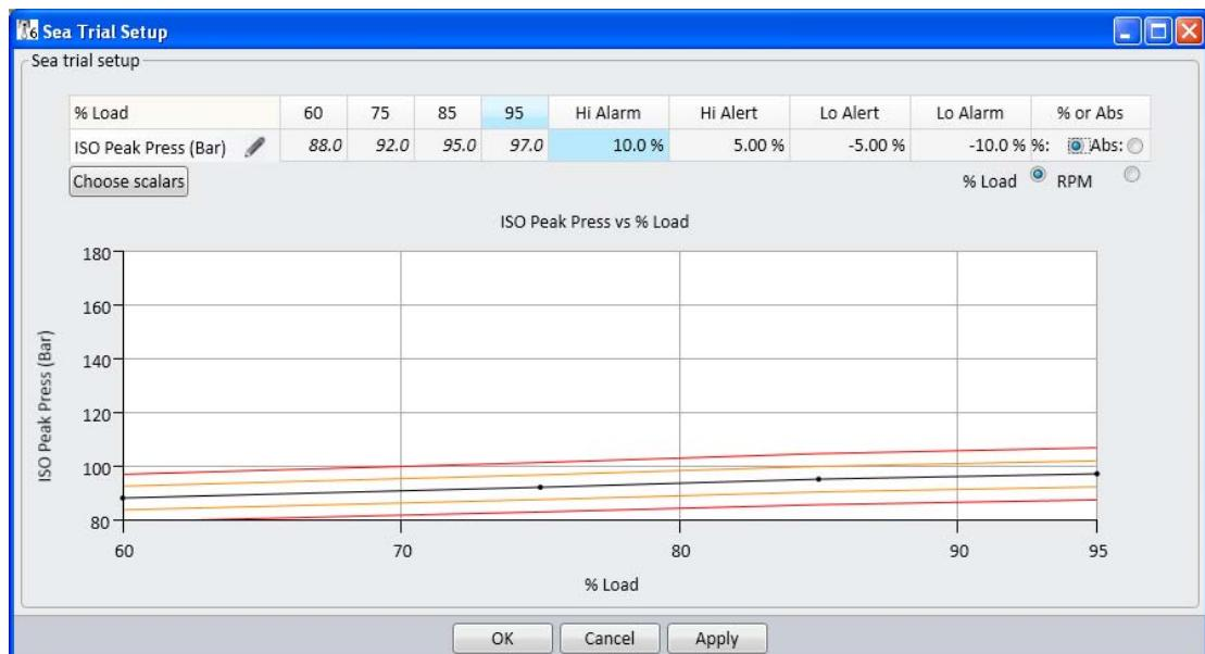
It is necessary to select high and low threshold levels for both alarm and alerts by clicking on the appropriate cell under *Hi Alert*, *Lo Alert*, *Hi Alarm* and *Lo Alarm* and entering either a % or an absolute figure. The *% or Absolute*
